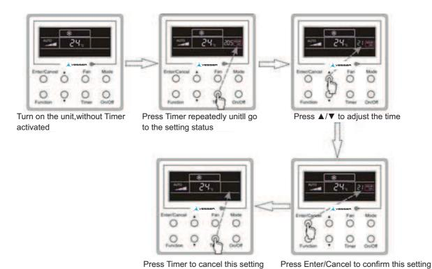
Fig.3.5.1 Timer off Setting under the "On" State of the Unit
