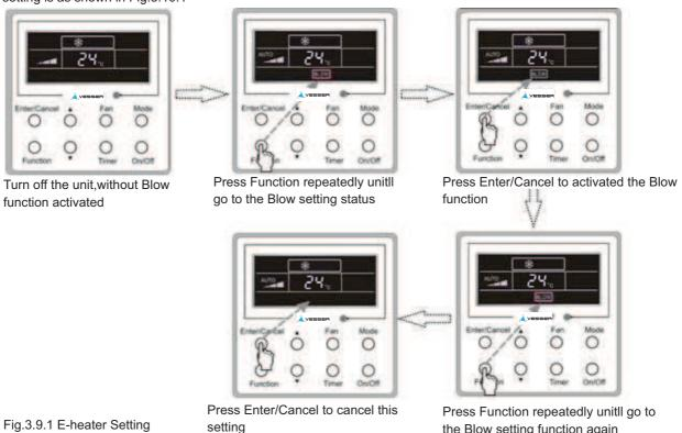
Fig.3.9.1 E-heater Setting
