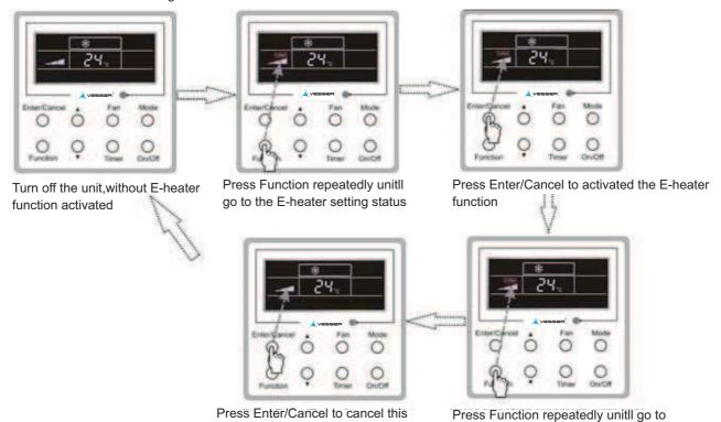
Fig.3.9.1 E-heater Setting
