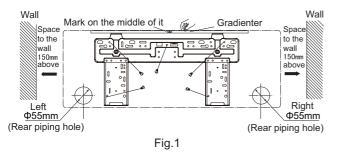
(2) Open a piping hole with the diameter of  $\Phi$ 55mm on the selected outlet pipe position.In order to drain smoothly, slant the piping hole on the wall slightly downward to the outdoor side with the gradient of 5-10°.(As show in Fig.2)
