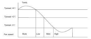
② Under FAN or COOL mode: if it is auto cooling mode or regular cooling mode, auto fan speed will be as follows:
