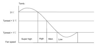
④ In this mode, set temperature will be automatically adjusted according to actual operation conditions.
